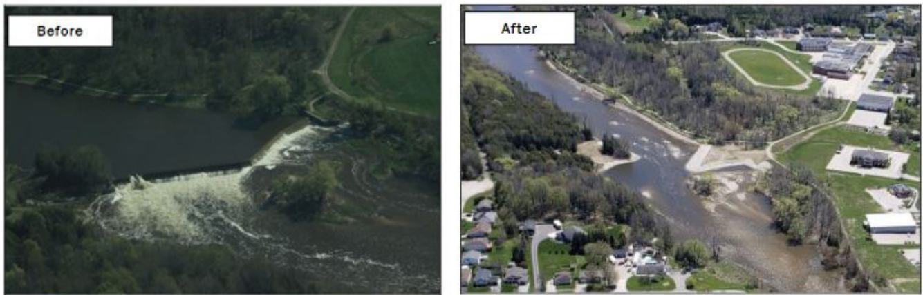
Figure 1 – Aerial images of the Truax Dam footprint, Walkerton, ON before and after removal. The original wooden dam was built in 1852 and later replaced by the concrete structure shown above in 1919. While the dam had a fishway that allowed the passage of some migrating salmonids under specific flow conditions, it posed a significant barrier to fish passage for more than a century before it was removed in the summer of 2019, restoring river connectivity.
